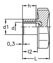
$\begin{array}{ll} D & = 50 \\ d1 & = 18 \\ d \ 6H = M10 \\ h & = 17 \\ L & = 31.0 \end{array}$
